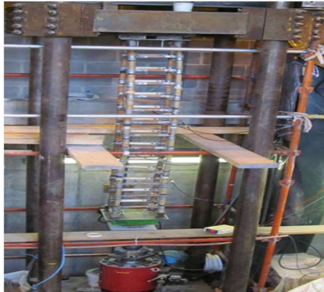
Figure 2.3 Banded column compression test (Kajjam et al., 2012)
