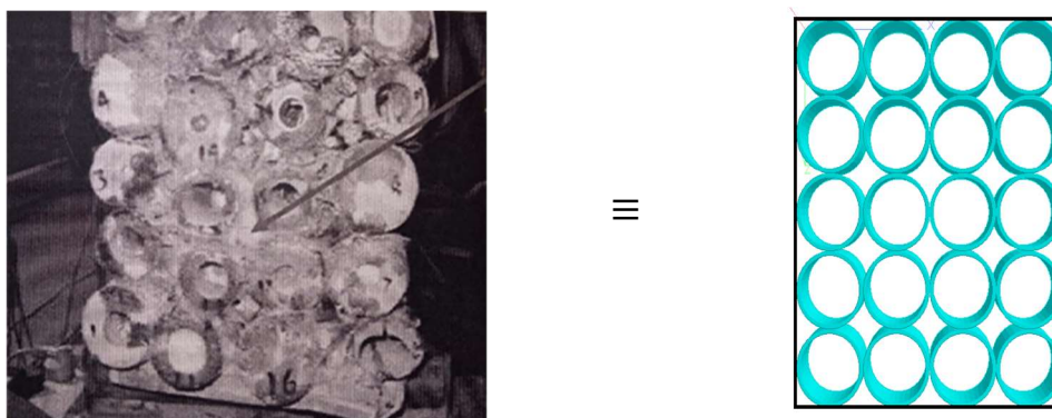
Figure 3.1 Cross section of the FRBC (Bhagat, 2017)
