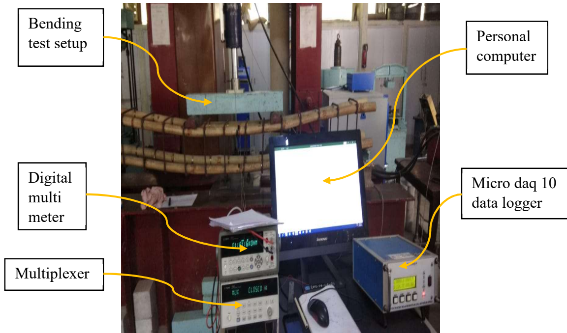
Figure 4.4 Four-point load test setup
