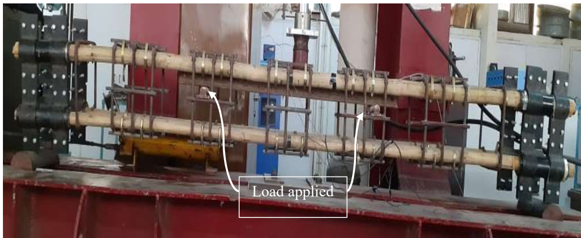
Figure 4.14 Full test setup with marking of load
