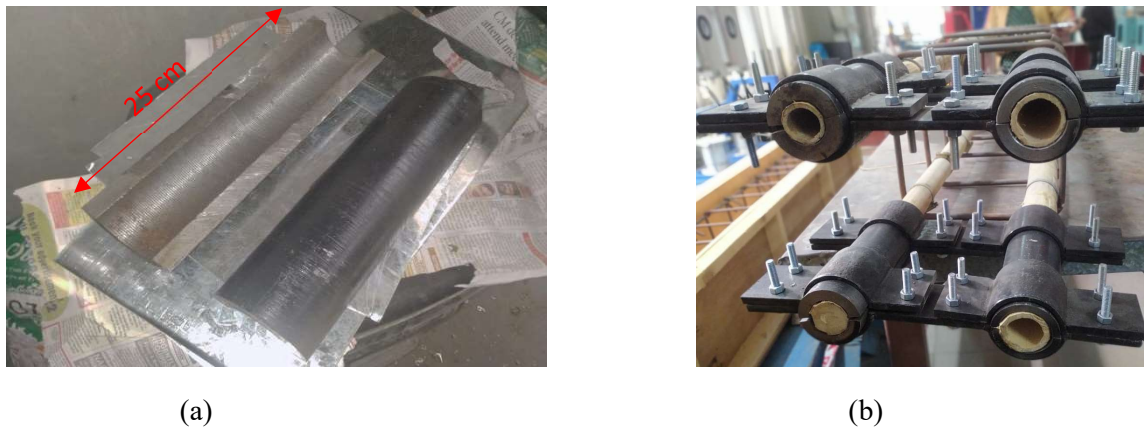
Figure 4.10 (a) Inner side threaded steel fixtures (b) Tightened fixture plate assembly with LBBS beam
