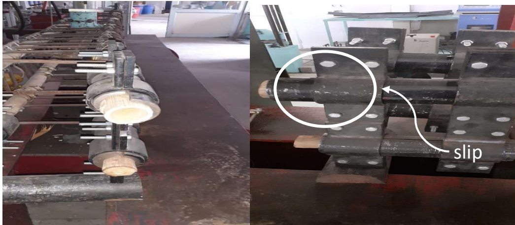
Figure 4.15 Slip was found after applying load
